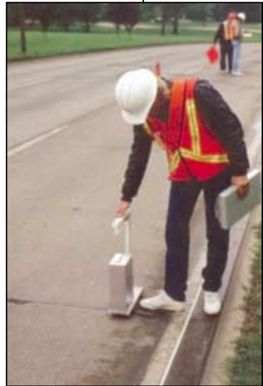
FIGURE B1 The Georgia Faultmeter in Use
